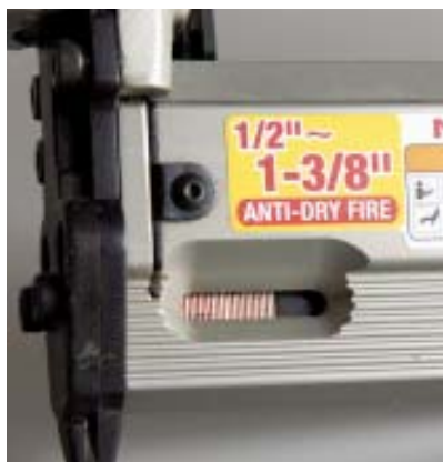
Figure 6. The better guns have a sizable indicator to let you know when to reload. Only the Max, shown here, has an anti-dry-firing mechanism.
