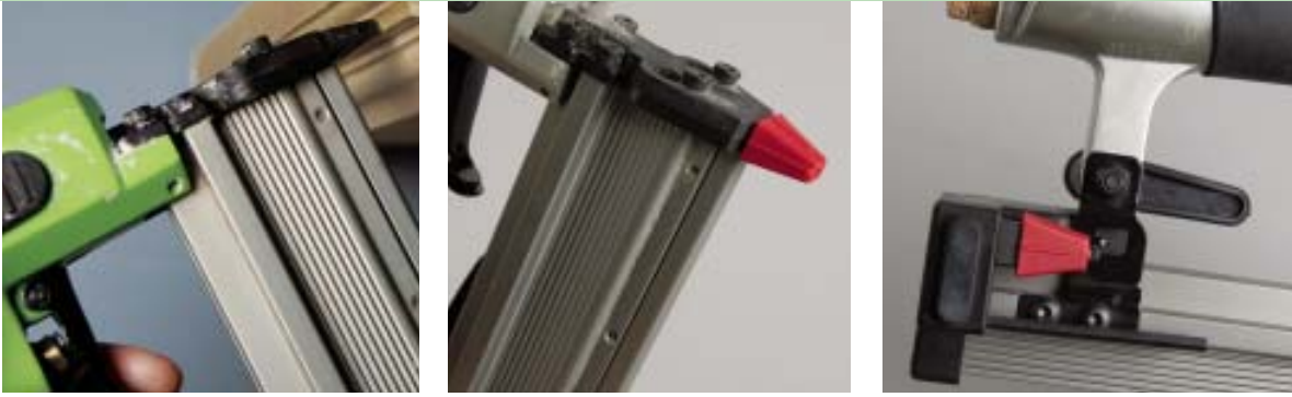
Figure 4. The most accurate pinners have small needle noses (left). Three of the guns — the Cadex, Grex, and Max — come with two rubber tips for protecting the work (center); the extra tip stores on the gun (right).
