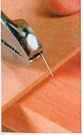
Non-stick router templates. You can use a pin nailer instead of double-sided tape to secure router templates to workpieces. Pins leave almost invisible holes in the workpiece when they're removed, but in most cases you can place them in spots that will be hidden.
