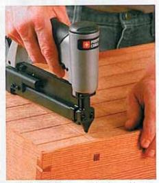
A bit of flex. Both pins and brads are thin enough to allow movement with changes in seasonal humidity, making them ideal for attaching back slats.
