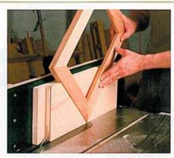
Quick work. Building this spline jig took minutes and it went right to work without a wait. Keeping the brads about 3 in. above the table prevents them from hitting the sawblade. The metal is soft, so striking a nail is unlikely to damage carbide-tipped tools. But flying shrapnel is a danger.
