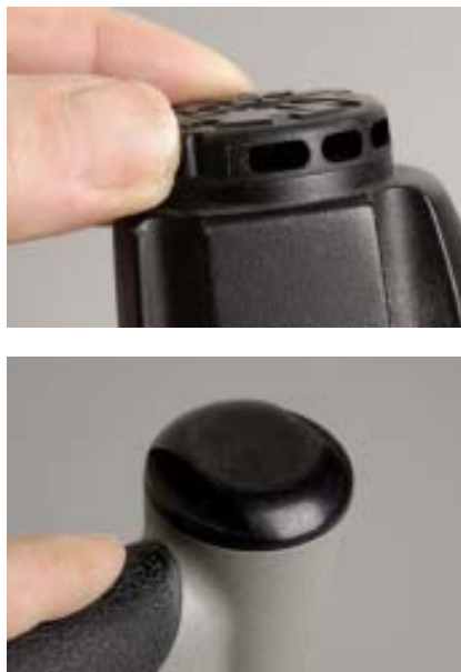
Figure 5. Several of the pinners have nonadjustable exhaust ports (left); the Nikle (above left) has a swiveling exhaust on the head. The author's favorite tools have a rear filtered exhaust (above), which completely dampens the blast of air.
