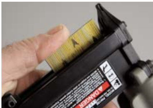
Figure 2. The Omer (above) and the Senco (above right) have slide adjustments for the different pin lengths. The Porter-Cable has a spring device that accommodates the various lengths: After inserting the pins (right), you press down to lock them into firing position (far right).
