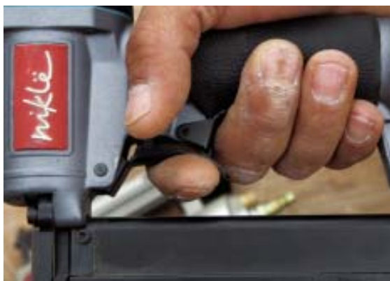
Figure 3. A good safety trigger (above) allows room for fingers on both the safety release and the trigger. Some designs (above right) make it difficult to engage the two triggers separately. The Nikle (right) allows hardly enough room to get your hand on the handle.
