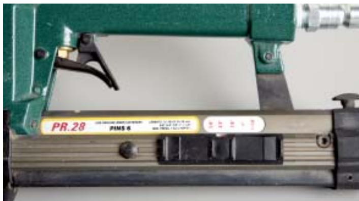
Figure 2. The Omer (above) and the Senco (above right) have slide adjustments for the different pin lengths. The Porter-Cable has a spring device that accommodates the various lengths: After inserting the pins (right), you press down to lock them into firing position (far right).
