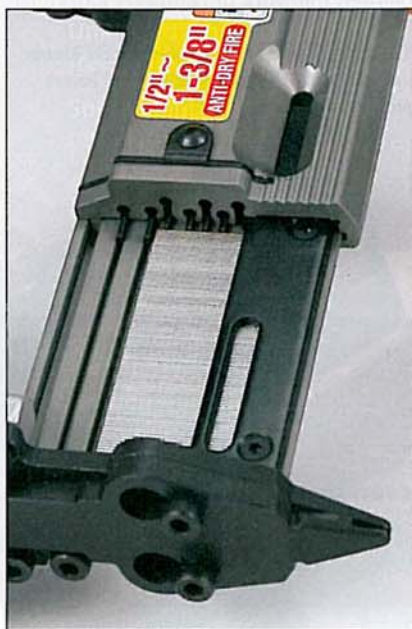
The Max pinner has spring-loaded guide pins typical of side-loading magazines and a large reload indicator window.
